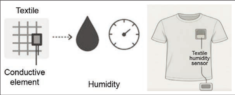
Fig. 3. Textile-based humidity sensor integrated into a wearable patch for real-time monitoring of moisture and physiological parameters [5]
